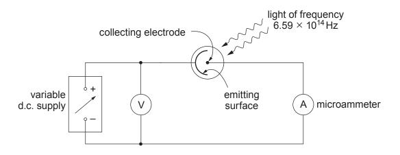
With zero pd applied, the microammeter indicates a current. At some pd between 0 V and  $0.35\,\mathrm{V}$  the microammeter reading drops to zero.
