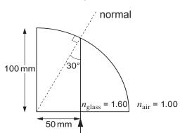
Calculate the angle of refraction into the air at the curved surface and carefully sketch the refracted beam **on the diagram**. [Use of a protractor is not required.][3]
