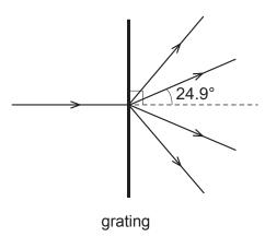
(i) First order beams emerge at angles of 24.9° to the normal (see diagram). Calculate the wavelength of the light.
